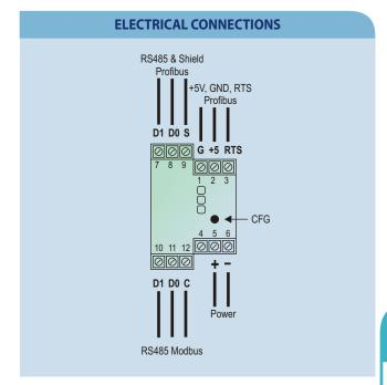
The product comes with a DB9 adapter to be optionally connected at the indicated pins, making the **DigiGate** connection available in the way recommended by the Profibus DP standard.
