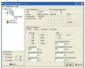
During the configuration process, the Modbus interface of the **DigiGate** will stop working as a master and start operating as a slave. In this condition, a computer equipped with a RS232-RS485 converter or a USB-RS485 is connected to the Modbus interface, and DigiConfig software will work as a Modbus network master in order to perform the **DigiGate** configuration.
