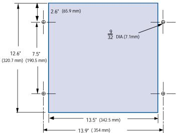
Panel cut-out for flush mounting
