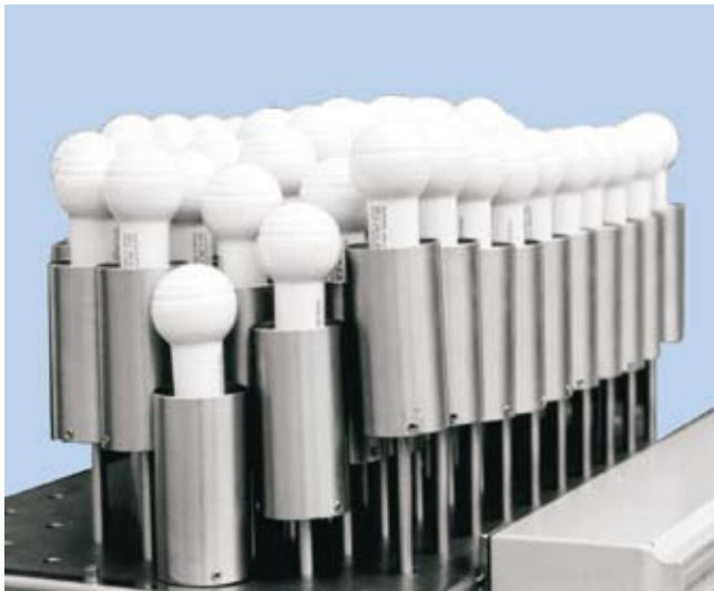
Figure 8: 3-D heating panel for laminating door trims
