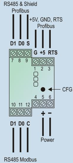
The product comes with a DB9 adapter to be optionally connected at the indicated pins, making the **DigiGate** connection available in the way recommended by the Profibus DP standard.
